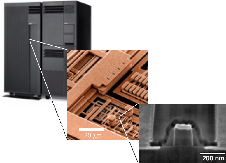
Figure 6.9. A computer integrates structure and function on many length scales. A transistor includes some layers of differentiated materials only a few atoms thick. However, our ability to impart structure at scales less than 180 nm is limited. In contrast, biological systems are richly structured all the way to the atomic scale.
